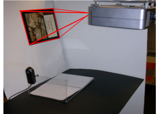
Using dual Photography We can simulate what a camera sees if it is put at the position of the projector.
